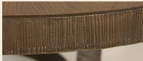
Detail of Hand Forged Texture created with an axe
